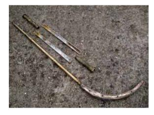
Hamble Propellers but despite their expertise it defeated even them. So it was decided to carefully slice the tube near the top and bottom without cutting the stock and then mill down the central section on both sides. To their credit the friendly guys at Hamble Propellers remained good humoured throughout this time consuming job, refusing additional payment beyond the modest quote they had given for the job at the outset.
