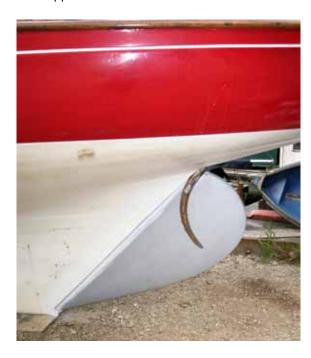
Since then the tiller has been held on with an M6 stainless steel bolt, assisted by Araldite to pack the tiller head very tight. This looked perilously underspecified but has proved perfectly reliable. Ideally a new stainless steel or bronze section should be grafted on the top of the stock, but that will have to wait until the next big job sees the rudder out again.
